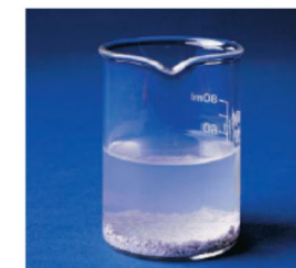
▲ \text{AgCl} does not dissolve in water; it remains as a white powder at the bottom of the beaker.
