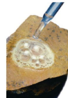
▲ Gas-evolution reactions, such as the reaction of hydrochloric acid (HCl) with limestone (CaCO 3 ), typically produce CO 2 ; bubbling occurs as the gas is released.
